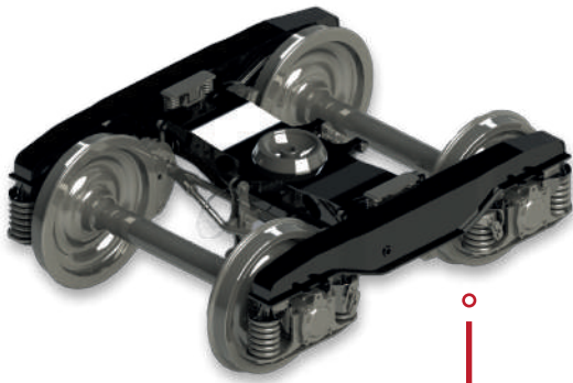
H-Type Bogie with Classical Brake System
