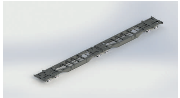
Sgss Light Type Container Wagon
